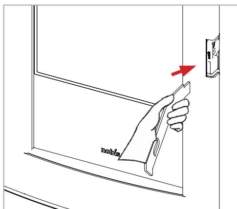
With a soft bristle brush, eliminate the combustion particulate, allowing it to fall in the slide beneath.
