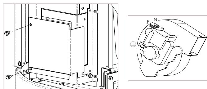
Make the electrical connection of the fan using the CANAL appendix, already present in the original wiring of the product. Live and Neutral can be inverted, unlike the earth connection (yellow / green colored cable) which must be connected to the earth of the fan.
