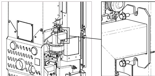
In the kit there is a cap with 3 screws of 8 for close the opening that allows disassembly of the hatch for cleaning the cast iron exchanger. The closure improves the heat exchange of the rear ventilation.
