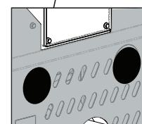
Position the stove canalization adapter by means of the 2 screws 5, present in the kit, and an 8mm hexagonal wrench.
