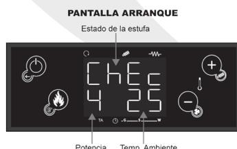
At this time, the electronic control board will perform a "ChEc" test on the heater, during which it will carry out a range of verifications. If the control board detects any anomaly, it will not start up and will instead give the corresponding error message. If everything is correct, the heater will begin the process of starting up.
