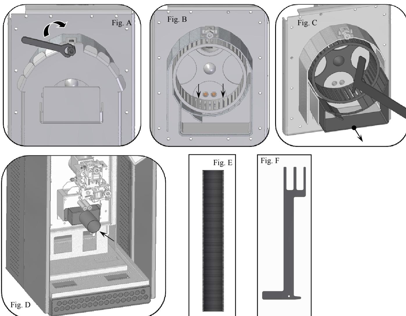
**⚠ ALWAYS KEEP THE HOLES OF THE ROTATING WHEEL CLEAN AND FREE OF ANY COMBUSTION RESIDUE. THE CLEANING FREQUENCY HAS TO BE APPROPRIATE TAKING CARE TO THE WORKING HOUR OF THE MACHINE AND TO THE CHARACTERISTICS OF THE COMBUSTIONS RESIDUE (HIGH PERCENTAGE OF ASHES OR PRESENCE OF DEPOSITS).**
