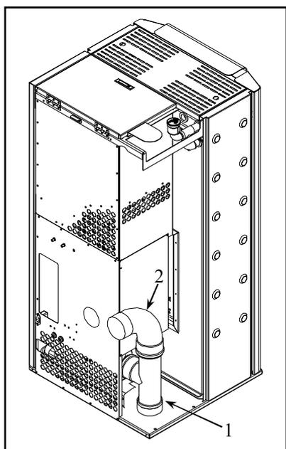
**Flue gas outlet on the upper side**
