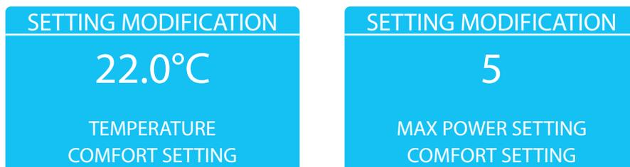
Use the **P4** key to switch from temperature to manual power and vice versa, use **P5/P6** to modify the values.
